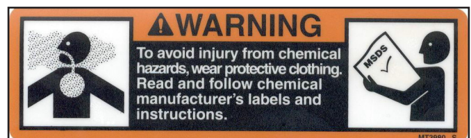
Figure 2: Chemical Warning Decal (DEMT3980) -Located on the main tank of the sprayer.
